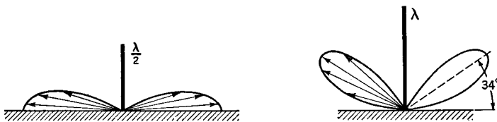
FIG. 8 E. Radiation patterns from vertical Marconi antennas
